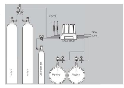
This means that if the analyzer is running several streams in a sequence the next stream to be analysed will be flushed automatically with a flush rate of approx. 0.7 - 1.1 SCF/hr. This is sufficient to flush at least 330 ft of 1/8" sample line.
