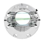
The reflective V paths interrogating the centre of the flow are sensitive indicators and enable the meter to be the "first to detect" dirt and grime deposited by process in the meter body. Conversely the direct paths provide extremely robust measurement under dramatic operating conditions typically seen in shale gas gathering points, coal seam, flare, wellhead and other harsh applications.
